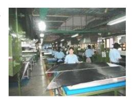
The sheets are cut to size and shape for hand lay-up.
